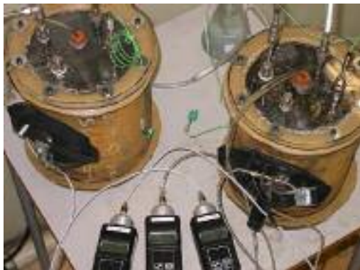
Full ring tests in progress with hydrogen Permeation probes. measurements.
